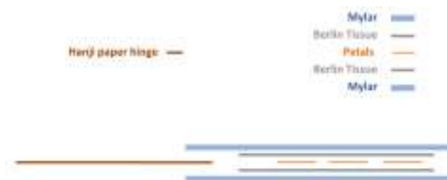
Fig. 20. Diagram of encapsulation assembly. The Berlin tissue is from Gangolf Ulbricht in Germany.
