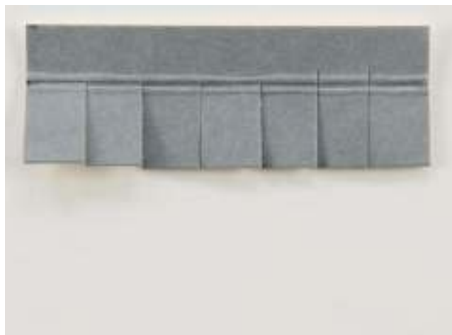
Fig. 17. Step 2: A strip is cut wider than the seal thickness, with the scored line running along it, and incisions are cut in the excess to allow the strip to bend.
