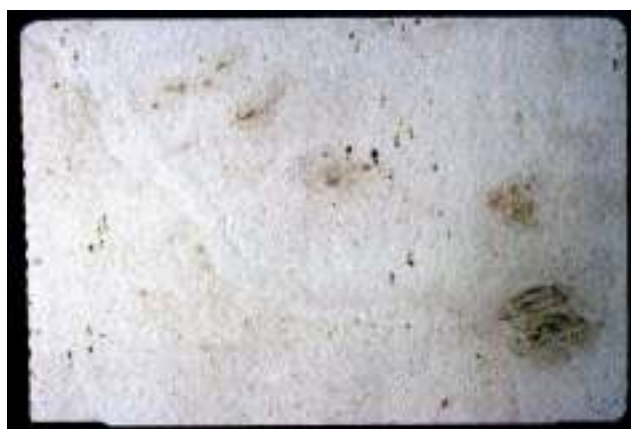
Fig. 2. The same detail of the lithograph’s verso after treatment, with the salts and accretions removed
