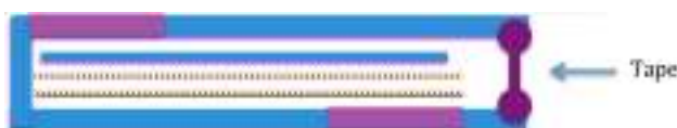
Fig. 27. The assembled package in cross section: note the tape at the edges.
