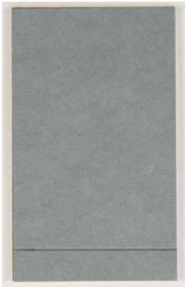
Fig. 16. Step 1: The folding box board is scored to the thickness of the seal (here, the distance between the bottom edge of the board and the fold line).
