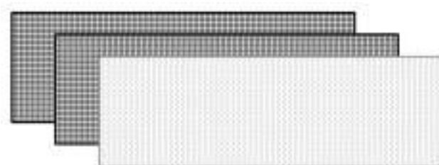
Fig. 26. The three layers of material to be placed inside the plastic channel: the layers allow the passage of air through the plastic to the suction device.
