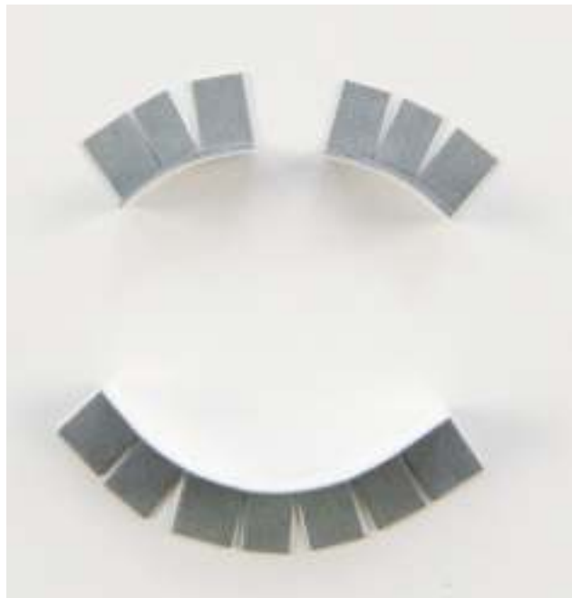
Fig. 18. Step 3: Tabbed strips are cut to length and bent to accommodate the shape of the seal.
