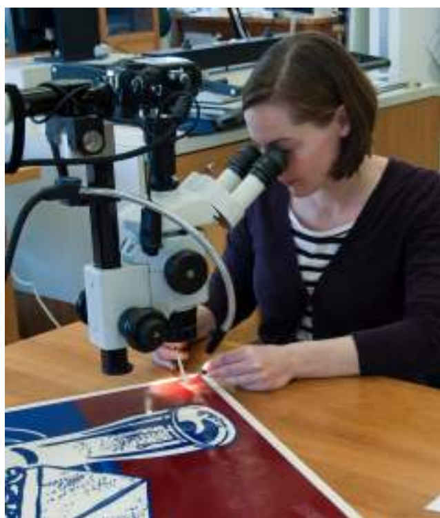
Fig. 3. Sampling the tape carrier under the microscope
