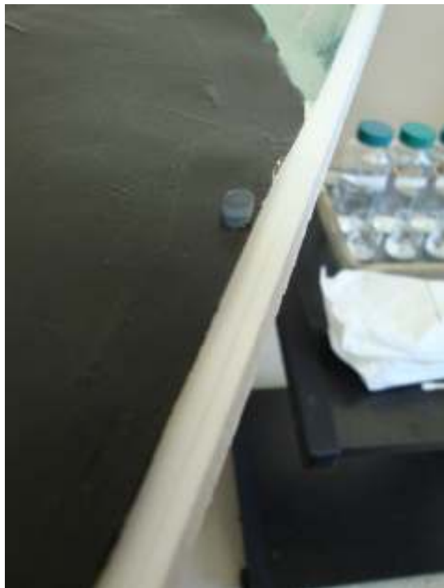
Fig. 1. An agarose pellet resting on the surface of an acrylic paint film
