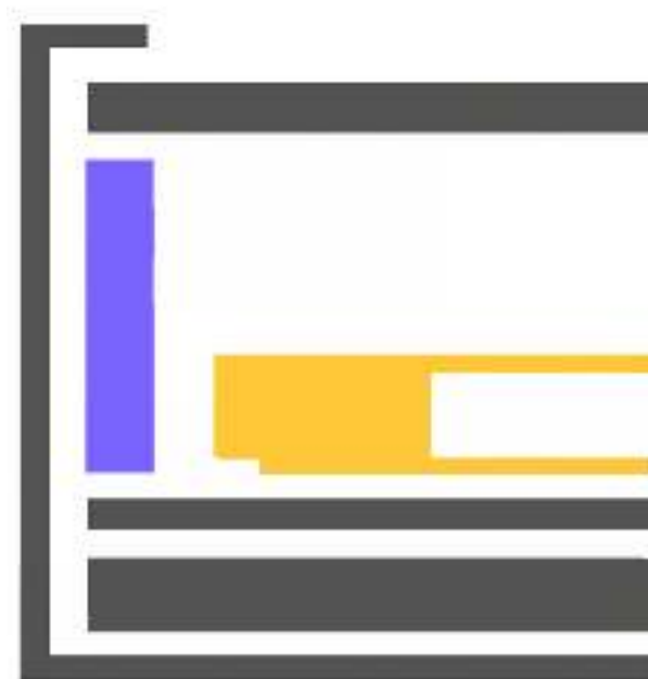
Fig. 15. Diagram of the layers of the housing package for Cassatt's The Pink Sash (Ellen Mary Cassatt). From top to bottom: glazing, tray sides around the pastel, rigid backing boards, and barrier film that wraps around to the front of the glazing
