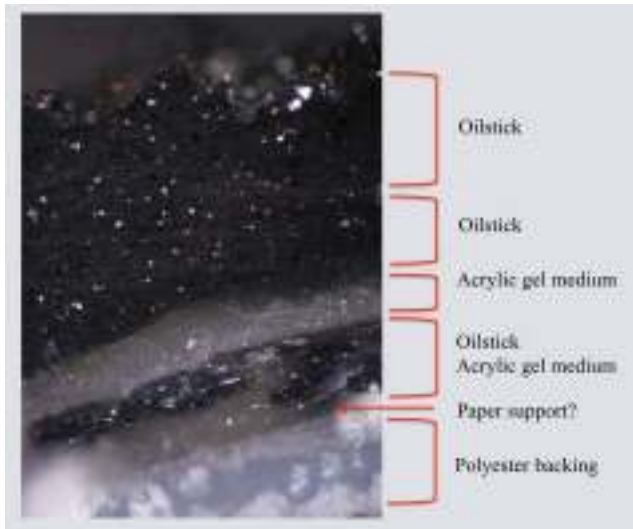
Fig. 3. Print cross section, visible light, polarizing light microscope. Composite of four images, each taken at 20x magnification. Print sample courtesy of Gemini G.E.L.
