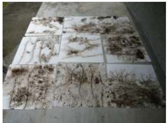
Fig. 1. Paper sheets after the gunpowder has exploded, before cutting
