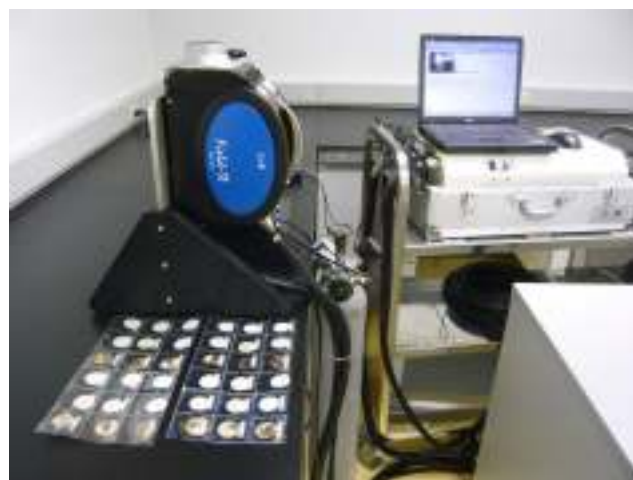
Fig. 5. Samples undergoing XRF analysis
