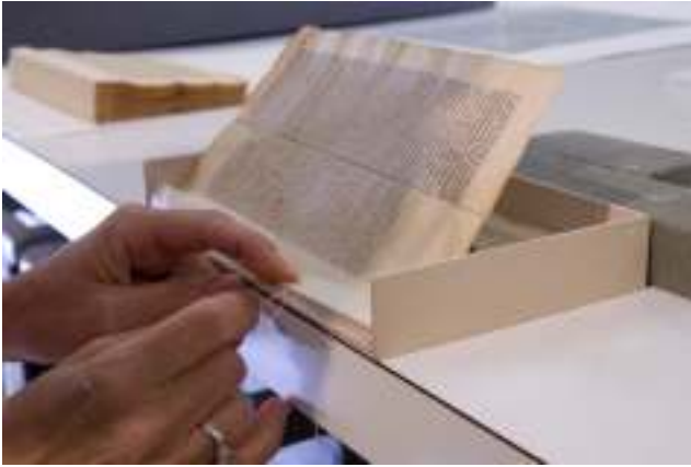
Fig. 7. Resewing the text block using a sewing tray made to the exact height of the desired thickness of the text block to align and protect page edges
