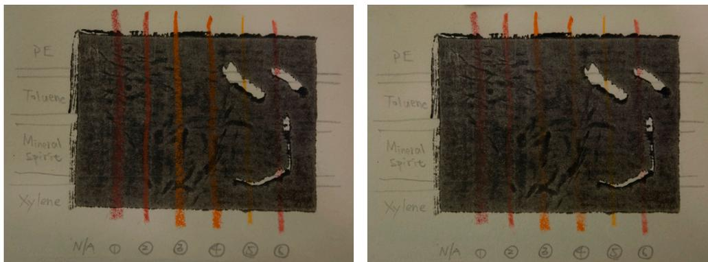
Figs. 9–10. Before (left) and after (right) mechanical cleaning
