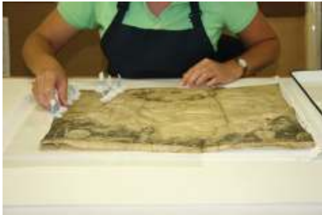
Fig. 6. Placement of rare earth magnets during tension drying, trial 1
