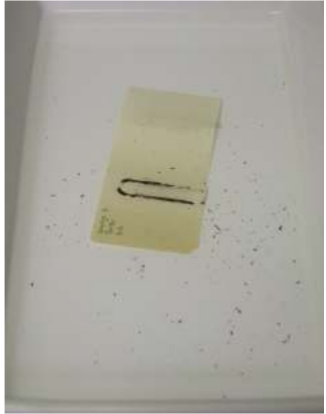
Fig. 16. Small black pieces of metal appeared at the bottom of the tray with sections treated with Sodium Dithionite. This observation was contrary to the corresponding sections treated with the Sodium Metabisulfite where the reduction of the rust caused the treatment solutions to turn a deep yellow color
