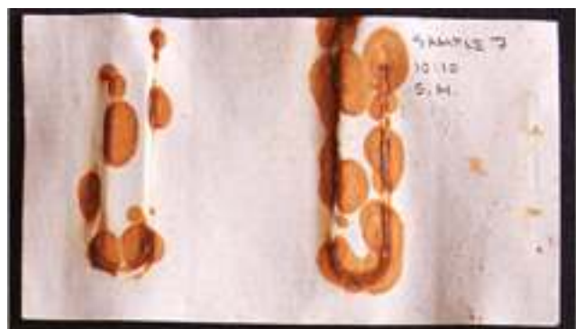
Fig. 9. Detail of a sample section after both rusted paper clips were removed
