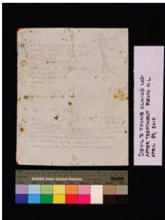
Fig. 3. Devil's Thumb climbing log after being treated in several consecutive solutions of equal concentrations of 10% Sodium Metabisulfite to EDTA. 21.1 cm x 24.9 cm. The Clausen Memorial Museum; Petersburg, Alaska
