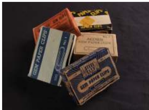
Fig. 6. Gem No.1 vintage paper clips, estimated seventy to eighty years old, purchased on E-Bay® to be used for creating rust in paper samples
