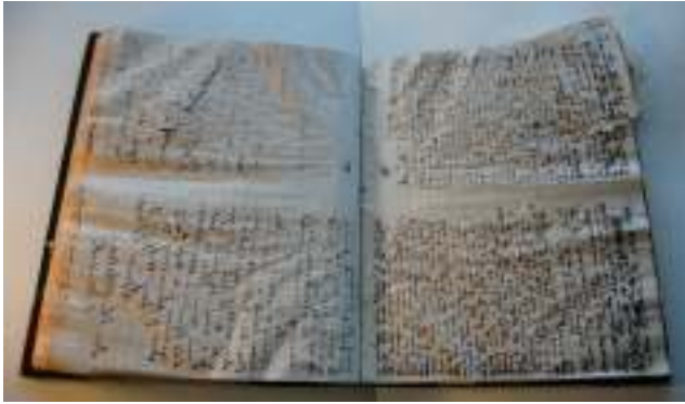
Fig. 3. Example of Baird copying book in poor condition, exhibiting severe iron gall ink corrosion
