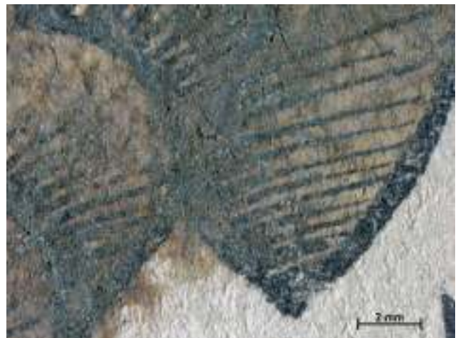
Fig. 6. Detail of the copper green pigment from a map in poor condition
