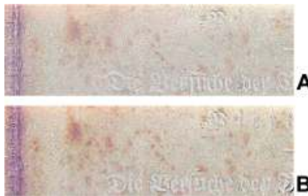
Fig. 6. False-color images showing the spatial variation of the effect of artificial aging on the spectral reflectance at three different wavelengths. Red channel: 710 nm; Green channel: 610 nm; Blue channel 450 nm. A) Difference image between 2 aging steps and no aging. B) Difference between 5 aging steps and no aging
