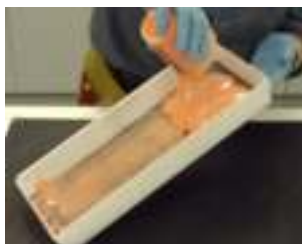
Fig. 2. The remainder of the silicone rubber is poured into the tilted tray.
