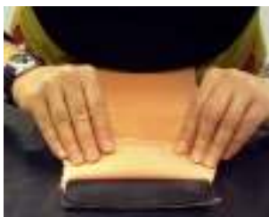
Fig. 3. The silicone mold is peeled away from the leather.
