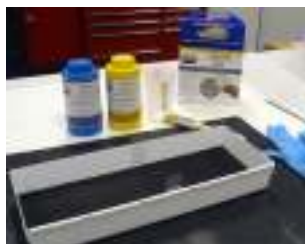
Fig. 1. Rebound® 25 Smooth-On Silicone Rubber components, walled plastic tray, and leather surrogate on prepared panel.
