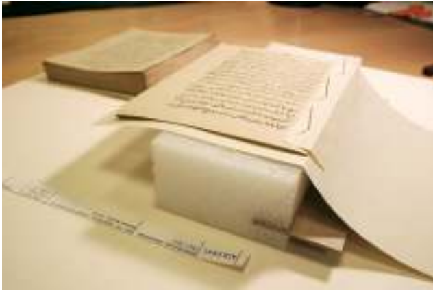
Fig. 5. Ethafoam sewing jig constructed to ease resewing of stab-sewn text blocks
