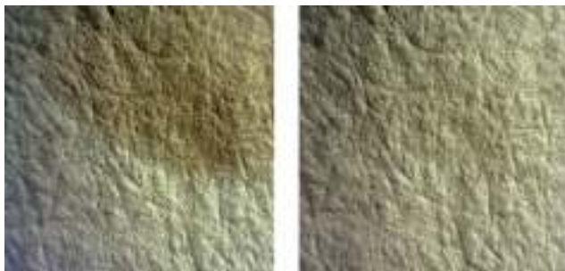
Fig. 21. A same piece of paper from 1635 before (left) and after treatment (right) with Gellan gel at 2% applied for 30 minutes. Images taken with Dinolite video microscope (65x)
