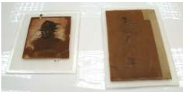
Fig. 29. The deacidifying gel positioned under the two drawings, using a sheet of Japanese paper as an interleaving tissue
