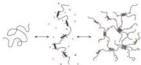
Fig. 13. Gellan gel coil-helix transition scheme. The stabilisation of the gel is caused by the presence of \text{Ca}^{++} ions. Image taken from M. Caggioni, P. T. Spicer, D. L. Blair, Rheology and microrheology of a microstructured fluid: The gellan gum case, in: "Journal of Rheology", 51-5 (2007) pp. 851-865
