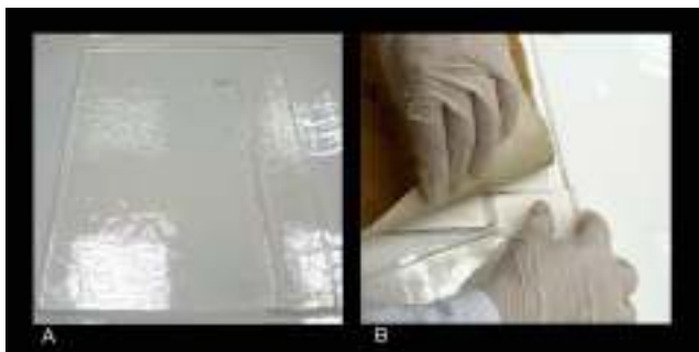
Fig. 28. An example of localised oxidation-reducing treatment: (A) a rigid oxidation-reducing gel and a simple rigid aqueous gel made according to a template; (B) positioning of the two gels under the drawing at the same time
