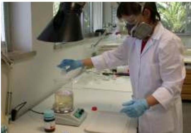
Fig. 27. The tert butyl aminoborane (7g/l) is added under the fume hood, when the hydration process of the Gellan is complete, using personal protective equipment
