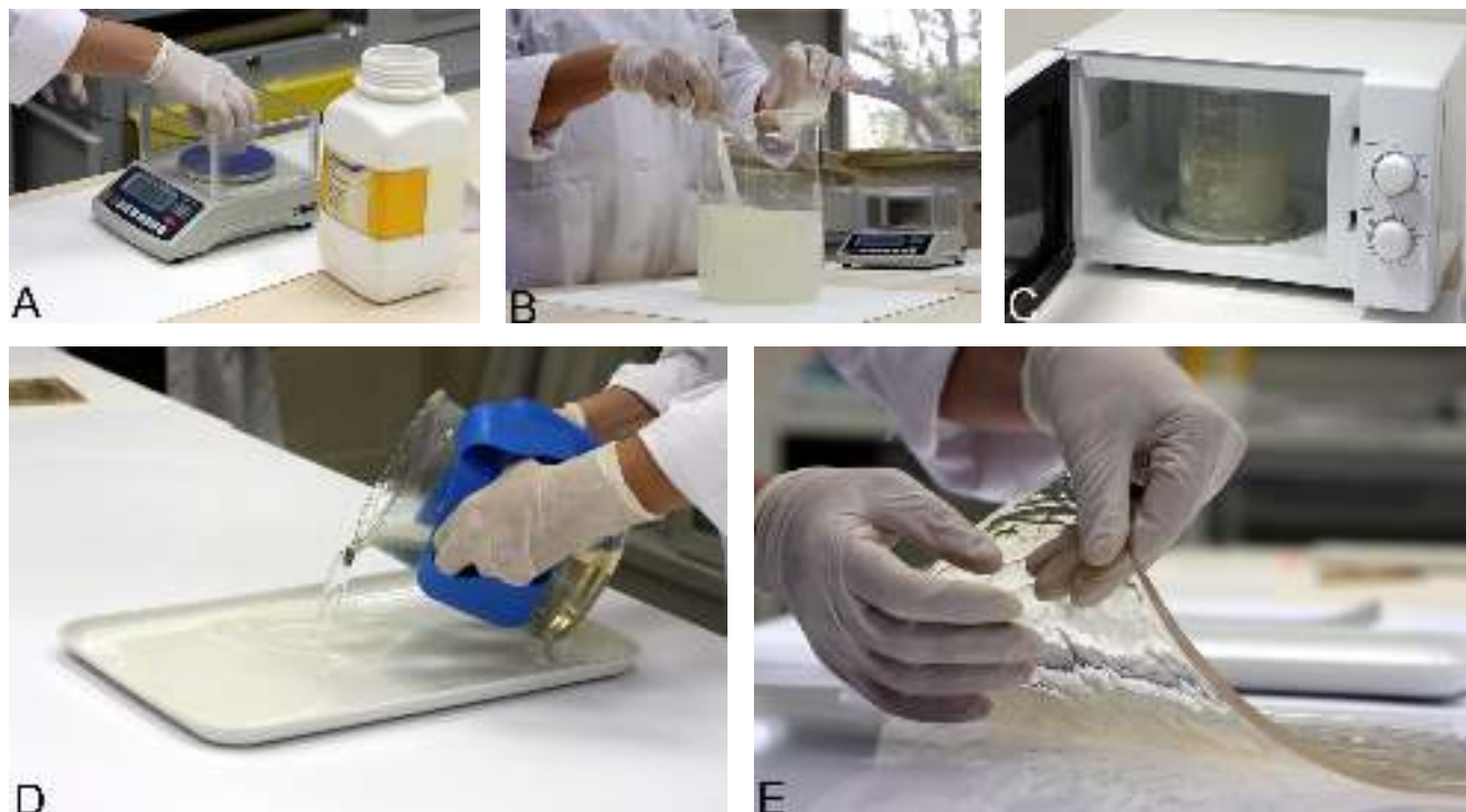
Fig. 16. (A) a saline solution of calcium acetate at low concentrations in deionised water (0.4g/l); (B) addition of Gellan powder to the saline solution; (C) the complete hydration of the colloidal dispersion is obtained by heating the compound to boiling point; (D) pouring of the solution in a basin (E) a gel obtained upon cooling of the hot solution
