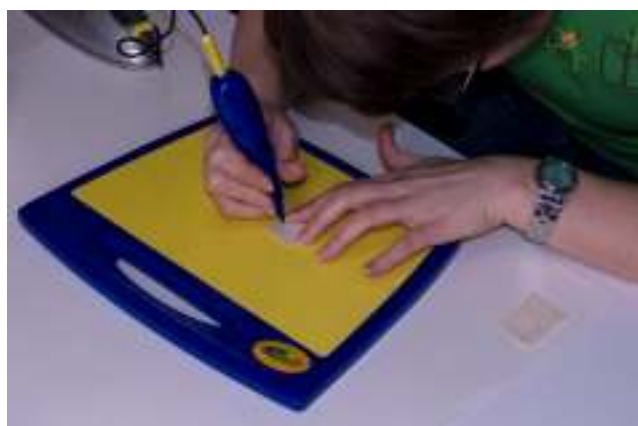
Fig. 8. Following the pencil line with the Crayola Cutter to create a perforated outline
