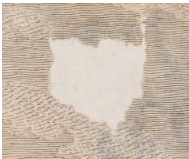
Fig. 11. A detail of the fill, recto. The edges of the fill were pared down and feathered further using water and a needle
