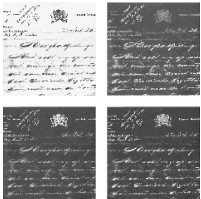
Fig. 6. Feature images calculated with the SDS algorithm: sub-strate (top left); print (top right); uncorroded ink (bottom left); and corroded ink (bottom right)
