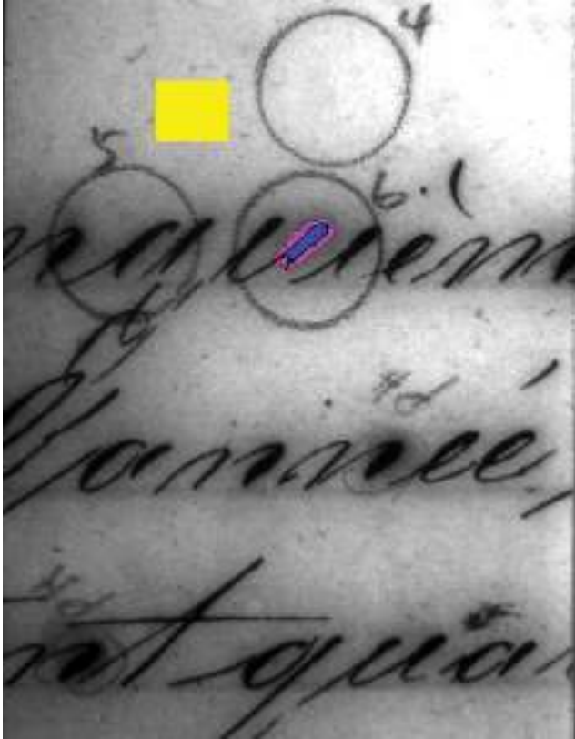
Fig. 6. An example of ink migration from a primary ink line as a result of high humidity exposure. Sample 6 untreated after humidity exposure (85% RH, 23° C; twenty-two weeks), three ROIs: yellow = paper; blue = ink; purple = migrated ink component
