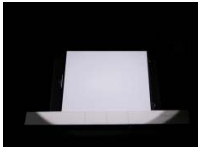
Fig. 3. The primary target (Spectralon) with the Recording Verification Target placed partially on top of it, in the position used for the recording of the document
