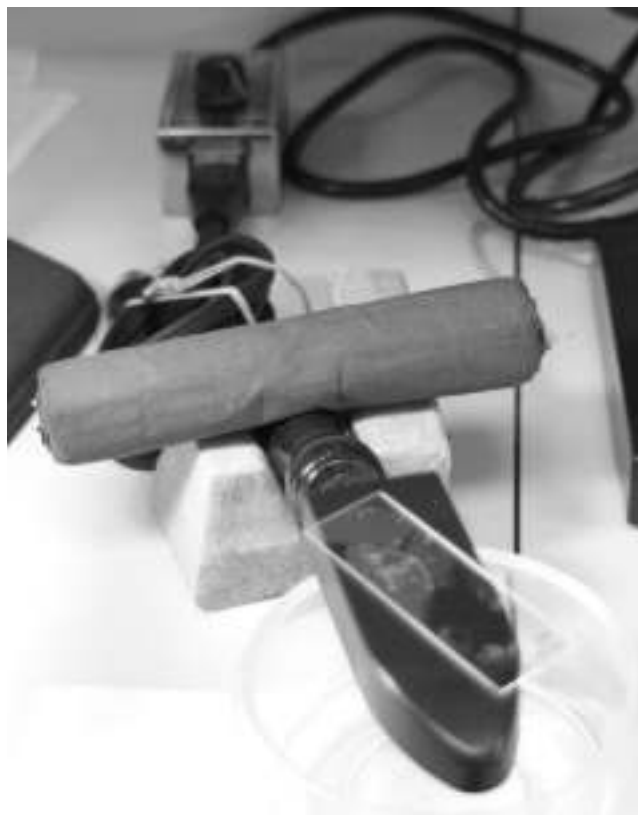
Fig. 1. The ninhydrin test setup using a tacking iron connected to a rheostat for heating the sample
