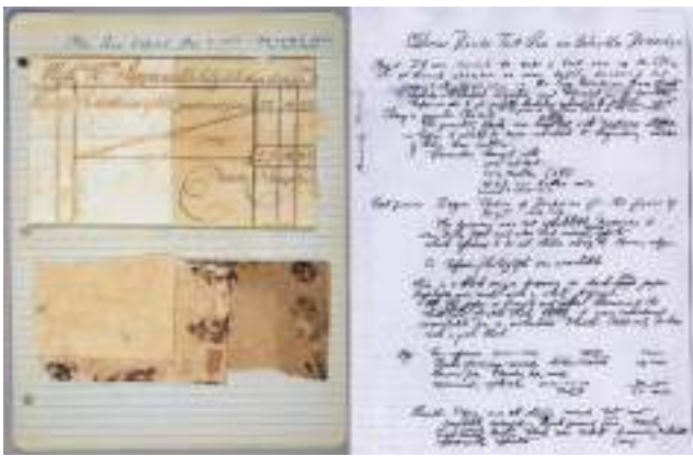
Fig. 7. Pages from Gettens's bleaching notebook: chlorine dioxide gas bleaching test on iron gall ink, May 7, 1951; chlorine dioxide gas test run on valuable drawings, May 15, 1951
