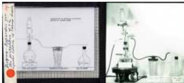
Fig. 3. Schematic drawing (left) and laboratory setup (right) for infusing water with chlorine dioxide gas. Courtesy President and Fellows of Harvard College
