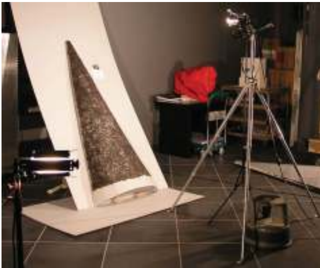
Fig. 13. Arched support used for photodocumentation of paper panels
