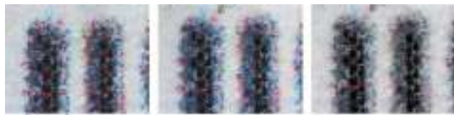
Fig. 3. Photomicrographs of printed black lines before (left) and after (center) fixing with Cartafix GS, and after immersion washing (right). Note the very slight bleeding of colored inks after fixing and slight fading after washing, while the black ink remained intact
