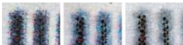
Fig. 4. Photomicrographs of printed black lines before (left) and after (center) fixing with Cartafix NTC, and after immersion washing (right). Note the marked bleeding and fading of colored inks after fixing and further fading after washing, while the black ink remained in place
