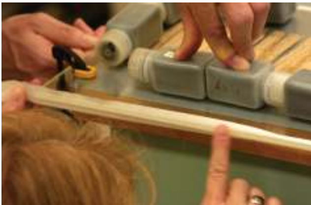
Fig. 8. Sealing with Filmoplast p-90
