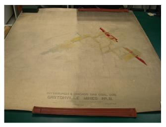
Fig. 8. The left side of this map was cleaned with soot sponges. The right half of the map shows the original amount of coal dust present
