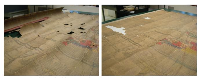
Figs. 12-13. Front of map before mending (left). Front of map after mending showing white muslin patches (right)
