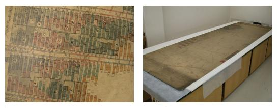
LEFT TO RIGHT Fig. 1. Detail of hardback mine map completed with watercolor and ink. The different colors and letters are date codes corresponding to the years that coal was mined out of the area
