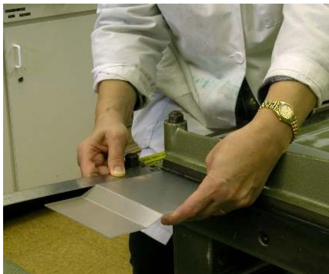
Fig. 2. To shape Vivak, clamp it in the board cutter . . .
