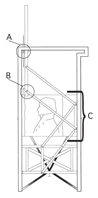
Fig. 1. Sketch of the physiognotrace used by Saint-Mémin. A -location of the sighting device, B - area of attachment of the graphite pencil, C - pantograph.
