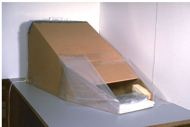
Fig. 6. Wind tunnel for drying the interleaved book. Box fan at the back is turned to pull air through.
