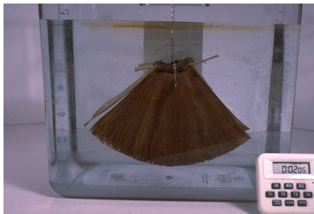
Fig. 2. Sewn text block fans out when suspended in the water bath
