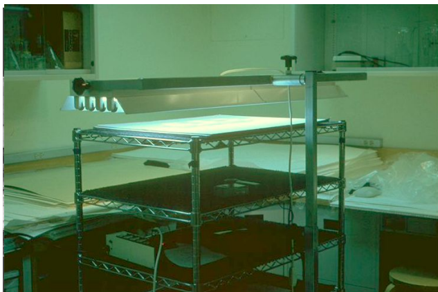
Fig. 6. Larger diazo test samples under light bank
