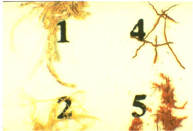
Fig. 14. Fiber samples at the various levels of deterioration (4X magnification)
