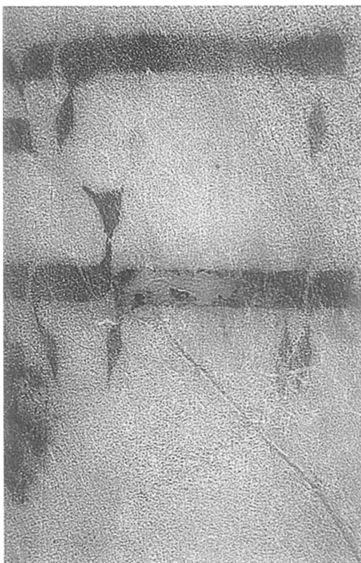
Fig. 28. Paper mend on verso of parchment sheet
