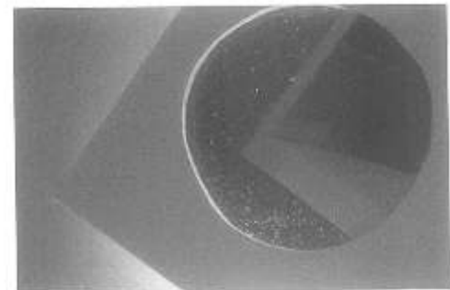
Fig. 6. Cellulose acetate film viewed through sandwich of polarizing filters
