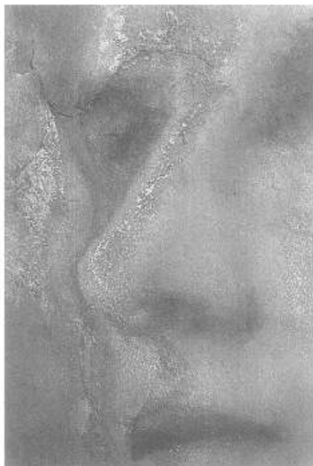
Fig. 11. Low detail of face showing an original mended tear with glue residue and paint damage
