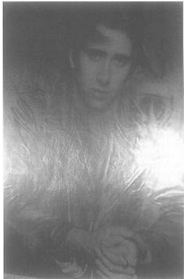
Fig. 2. Dye diffusion thermal transfer print in specular light
