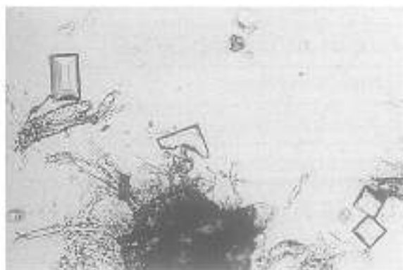
figure 7. Crystals of \text{NH}_4\text{MgPO}_4 \cdot \text{H}_2\text{O} associated with paper fibers viewed at 200x. The crystals resemble envelopes or tiny rooftops.
