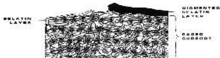
Fig. 4. Line drawing based on Figure 3. The gelatin print transfer sits on the surface of the gelatin-coated transfer paper and the shadow/highlight interface is visible as a cliff-like drop off.
