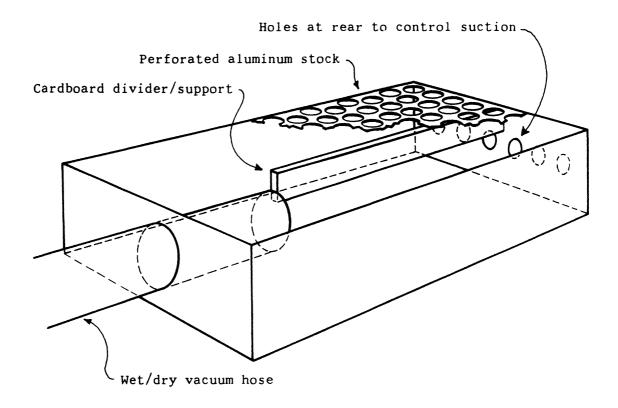
Fig. 1. Small suction box design (cutaway drawing)
