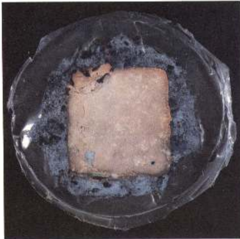
Color pl. 6. White lead sample on a cast rag paper colored with Prussian Blue pigment. Orange discoloration appeared at the edges of the sample after five days exposure to hydrogen sulfide.
