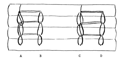
Unsupported structure. Chain pattern across spine; in-line, periodic fold pattern. There are four sewing stations - A is at the head and D is at the tail. Two needles are used, each sewing between two stations - A & B or C & D. They sew independently but identically. Enter at A, continue-on to B, exit, drop to-the-outside, link, climb, enter at B, reverse, exit at A, drop to-the-outside, link, climb, change-over and enter at A in the next section.
