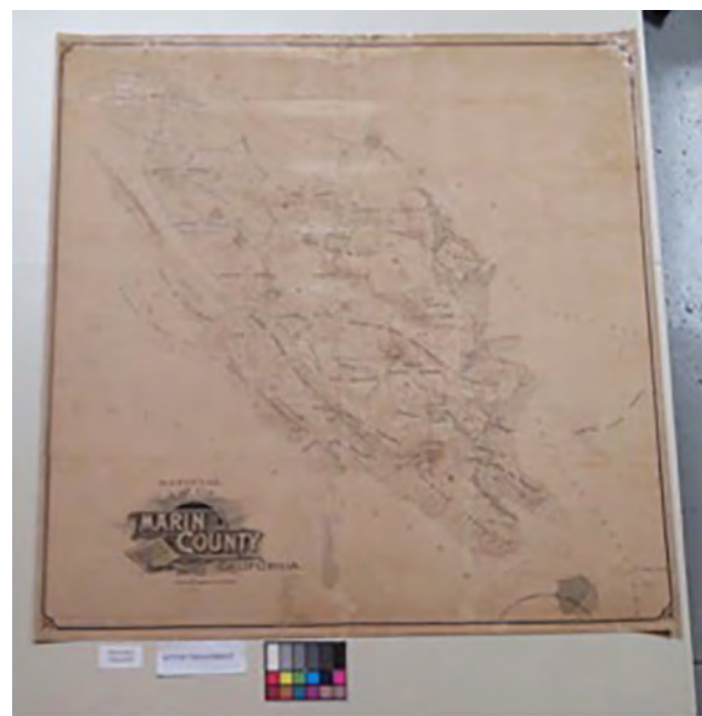
Fig. 6. 1892 map of Marin County. Completion: backed with one layer of medium-weight Sekishu and wheat starch paste. Stretch-dried and flattened under felts and weight. Once completely dry, residual varnish was reduced/removed with fine sandpaper. Losses were filled with toned paper and narrow strips of similar toned Japanese paper wrapped around the margins, applied with paste. To be framed.
