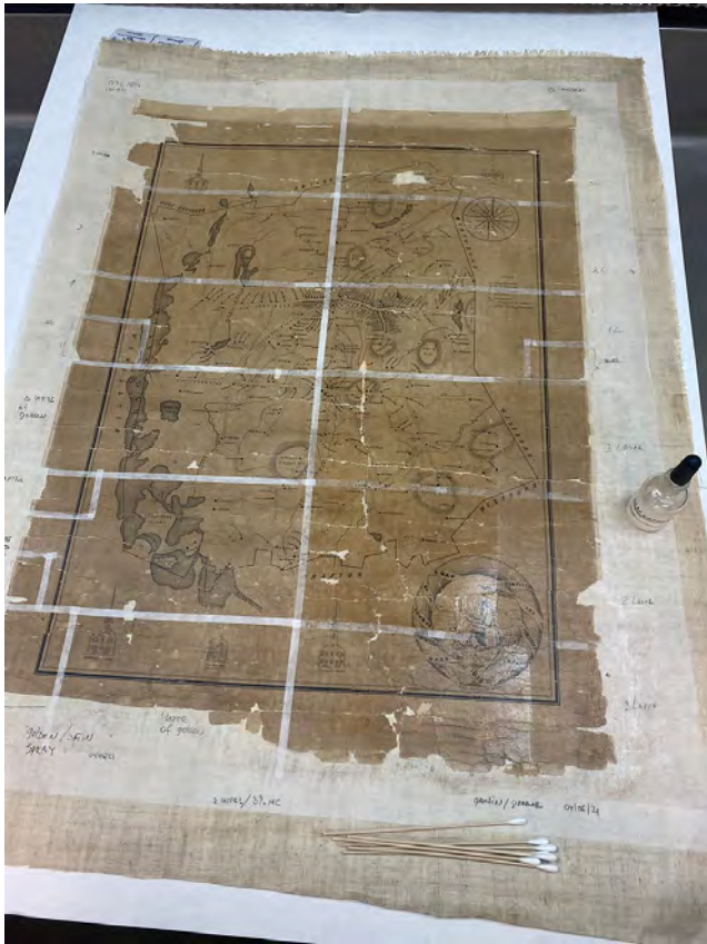
Fig. 5. Map sample testing permeability and reversibility over a larger area. Clockwise from upper left: 10% B-72 in ethanol, 5% Crystalac #500, Gambin Gamvar, and Golden Archival Varnish.
