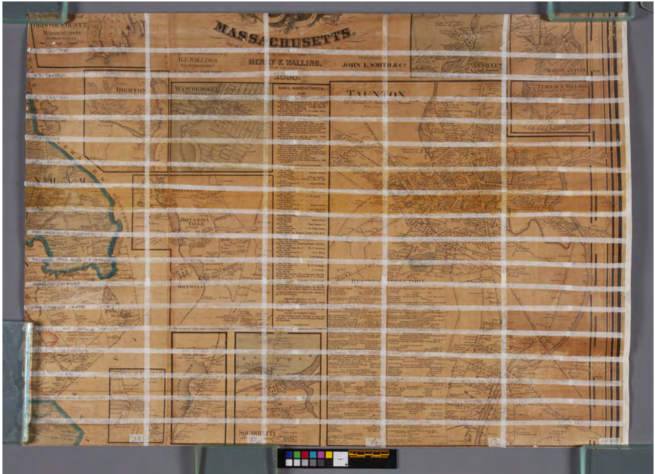
Fig. 2. Wall map test sample with all coating options. From left to right, samples are over 3% methylcellulose, 2% methylcellulose, 4% methylcellulose, 5% methylcellulose, and the control section (no isolation layer).
