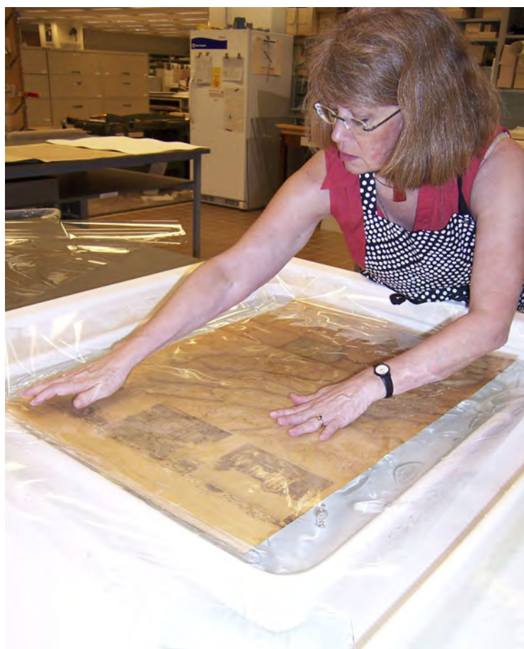
Fig. 2. Map section in alpha amylase solution between two sheets of clear polyester film floating over a tray of warm water.
