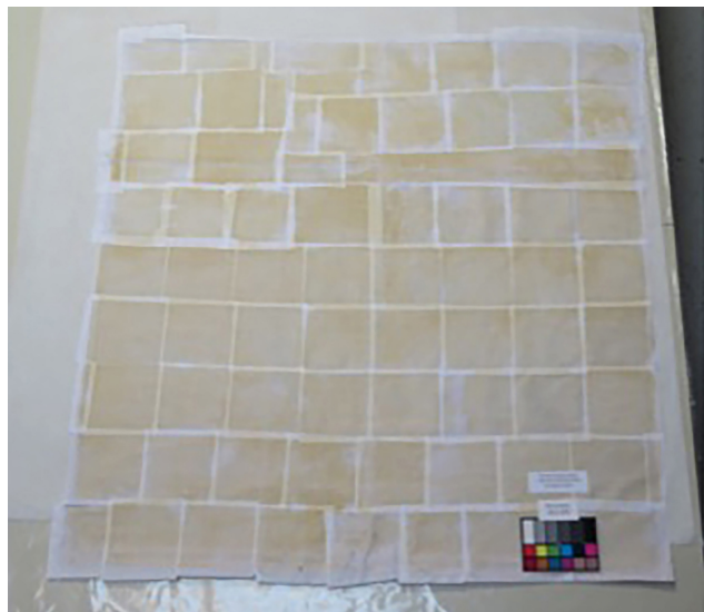
Fig. 3. 1892 map of Marin County. After application of rayon facing with a thin paste wash. Dried under Hollytex and felts.
