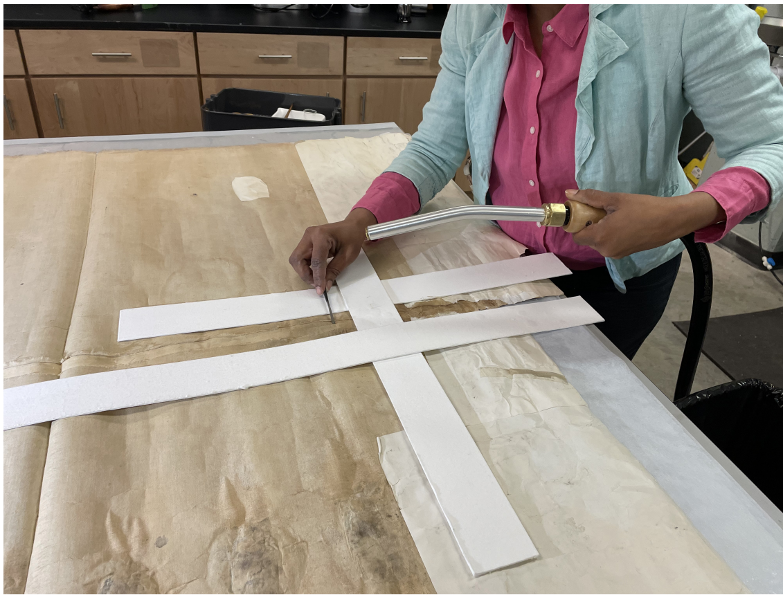
Fig. 5. Valinda Carroll using a Jiffy Steamer to separate the map panels.
