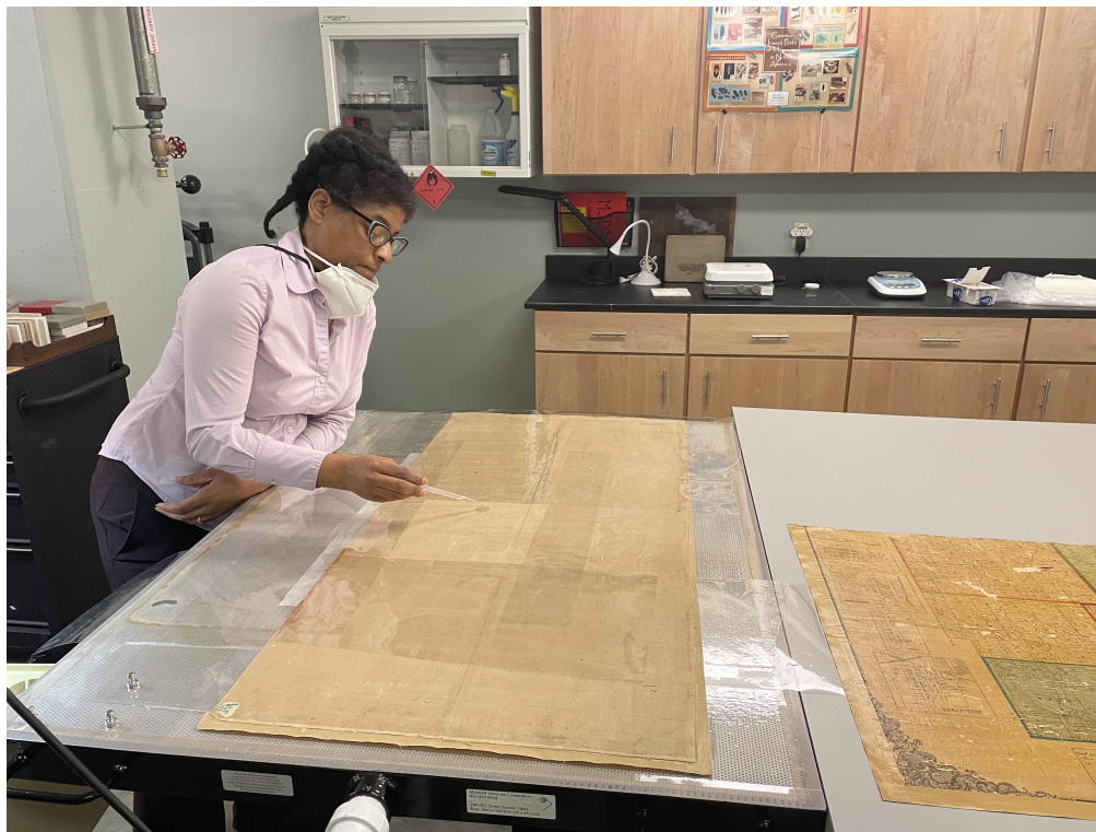
Fig. 4. Valinda Carroll conducting a varnish removal test on the suction table.
