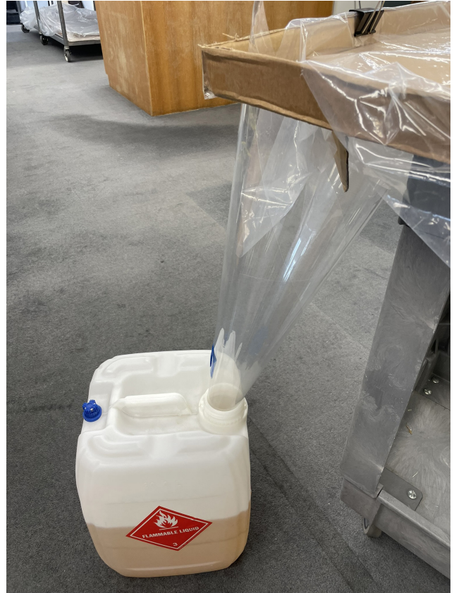
Fig. 6. Draining the sink by pushing the plastic through the hole to a Mylar funnel. Courtesy of CCAHA staff.
