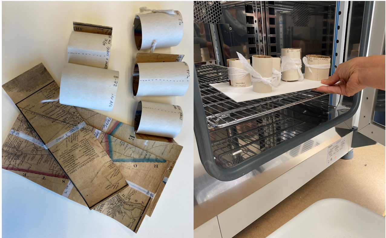
Fig. 3. Finalist coatings prepared for further testing (left) and being placed in the baking oven (right).
